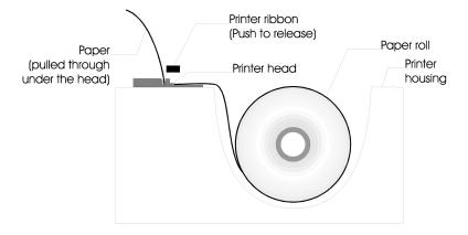
Feed the free end of paper into the printer through the metal slot beneath the printer ribbon. Start the paper feed sequence until the paper has emerged from the top of the printer, feed the loose end through the cover and refit.
