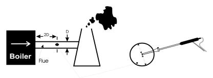
The probe depth stop cone provided with the instrument allows the probe to be used in holes whose diameters range from 8 mm to 21 mm (5/16 to 4/5 inch).
