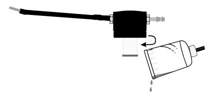
Carefully remove the end cap from the in-line housing. Dispose of the condensate in a suitable drain; care must be taken, as it could be acidic. If condensate spills onto the skin or clothing, clean off immediately using fresh water and seek medical advice if problems occur.
