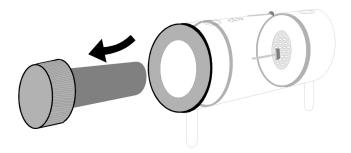
Remove the end cap from the filter housing. Carefully remove the paper filter element and dispose of it. Clean the inside of the filter housing with a suitable soft cloth. Insert a new filter element onto the spigot on the filter end cap and carefully insert it into the filter body.
